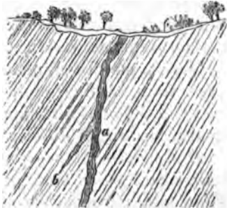
FIG. 7.—True vein, a , sending out a branch, b , corresponding with bedding.
